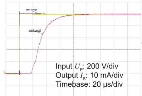
Figure 6: Typical step response (0 to 1000 V)
